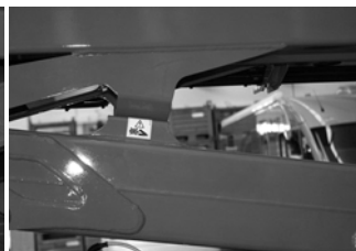
Fig. 95 Example potential shearing risk zone 3
