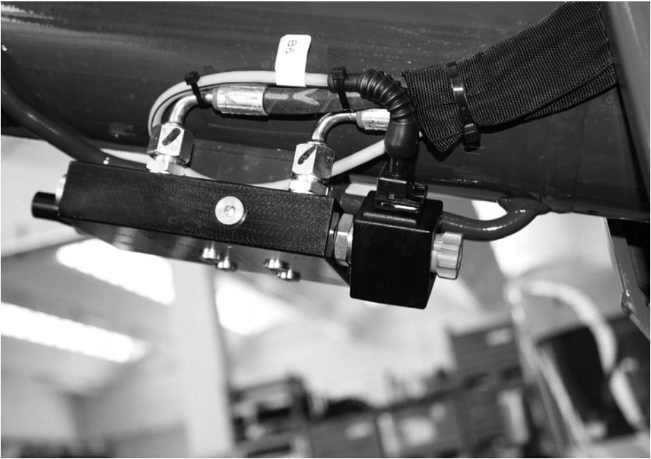
Fig. 65 Solenoid valves for emergency descent
