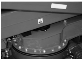
Fig. 94 Example potential shearing risk zone 2
